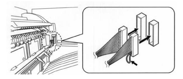
Please be sure that those two connectors are inserted into the appropriated jack. (13-pin connector should be left and 12-pin with a short line be right).
